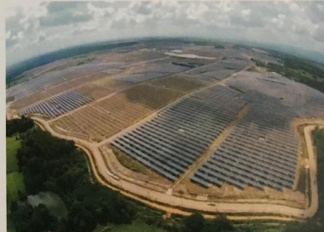
Installation Site: Thailand Project: 80MW Flat Single Axis Solar Tracker
